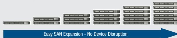
**Need more server or storage ports? Simply add another switch to the stack—no need to move existing cables or disrupt devices.**
